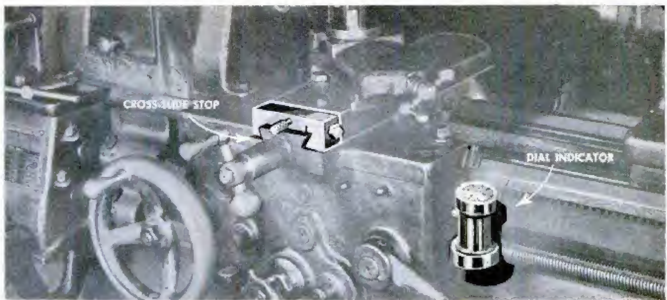
Dial indicator and slide stop speed up accurate thread cutting in lathe. Note position of the parts
